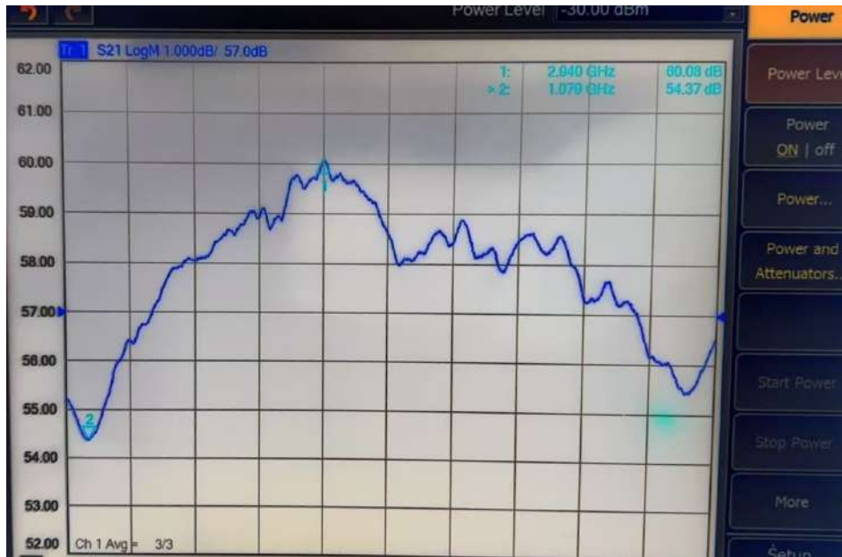
Figure 1: Gain Flatness Test Result
