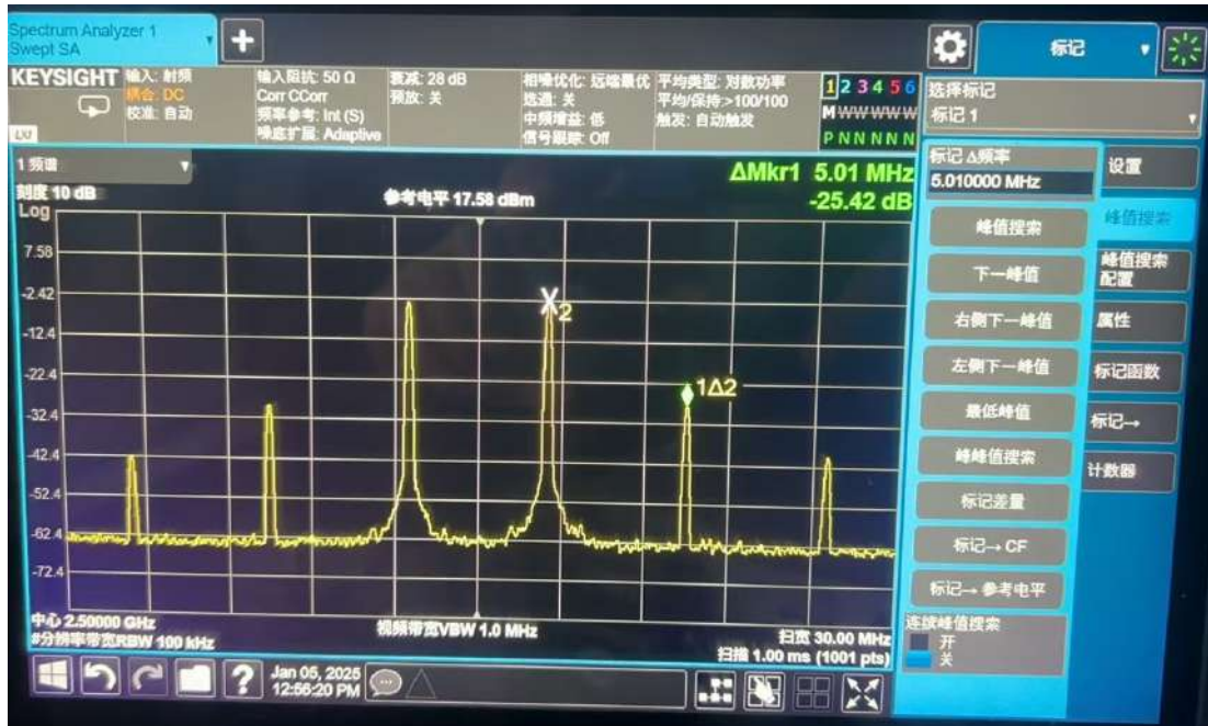
Figure 30 2.5GHz IMD3 Test Result
