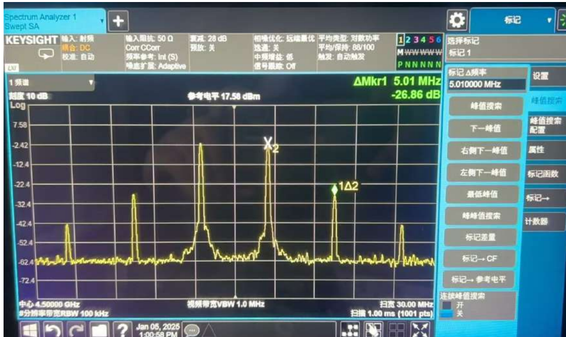
Figure 34 4.5GHz IMD3 Test Result
