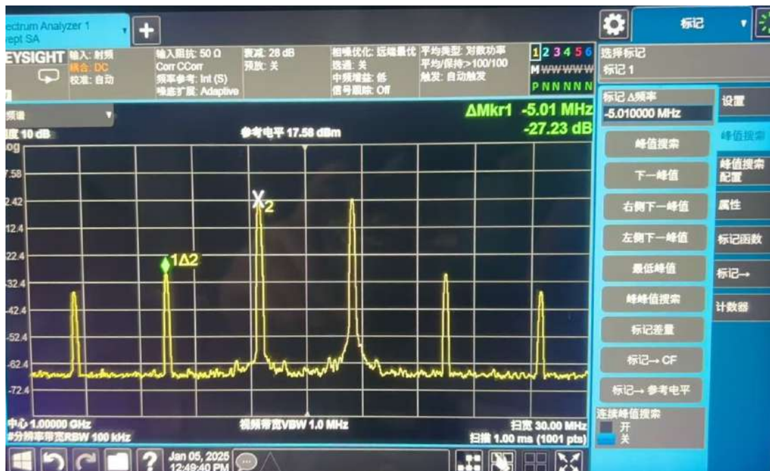
Figure 27 1.0GHz IMD3 Test Result
