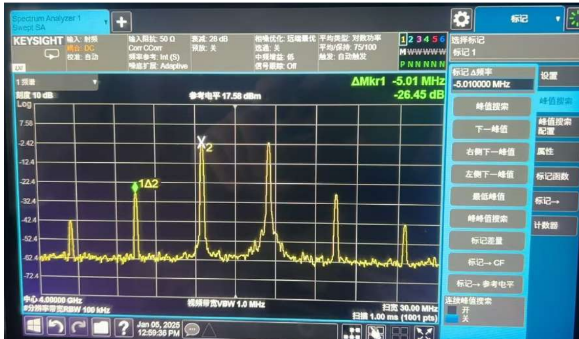
Figure 33 4.0GHz IMD3 Test Result
