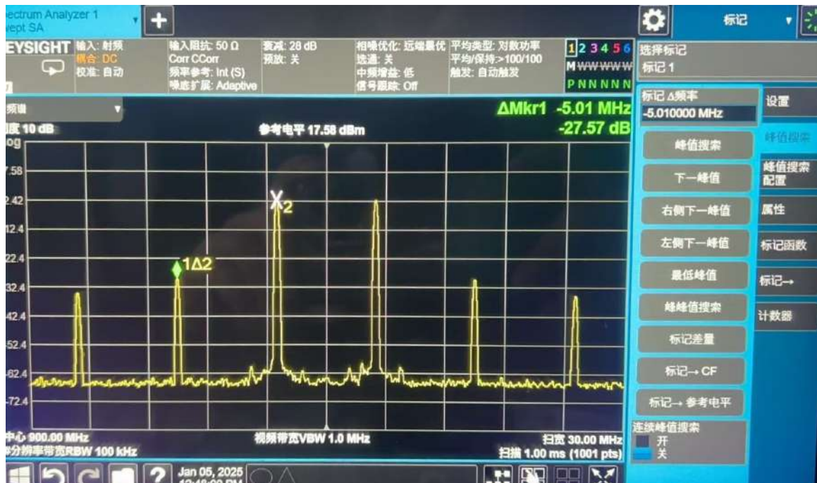
Figure 26 0.9GHz IMD3 Test Result
