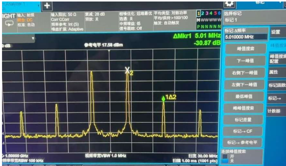
Figure 28 1.5GHz IMD3 Test Result
