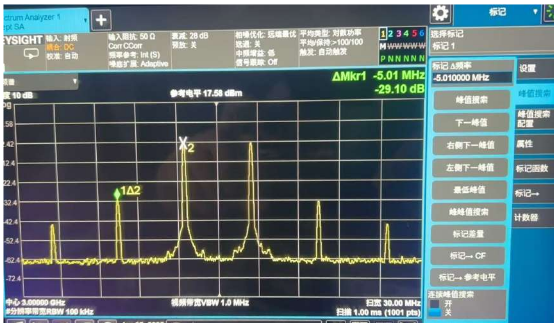
Figure 31 3.0GHz IMD3 Test Result
