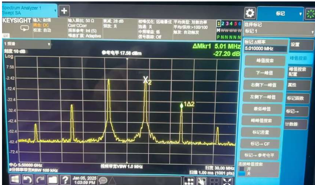
Figure 36 5.5GHz IMD3 Test Result
