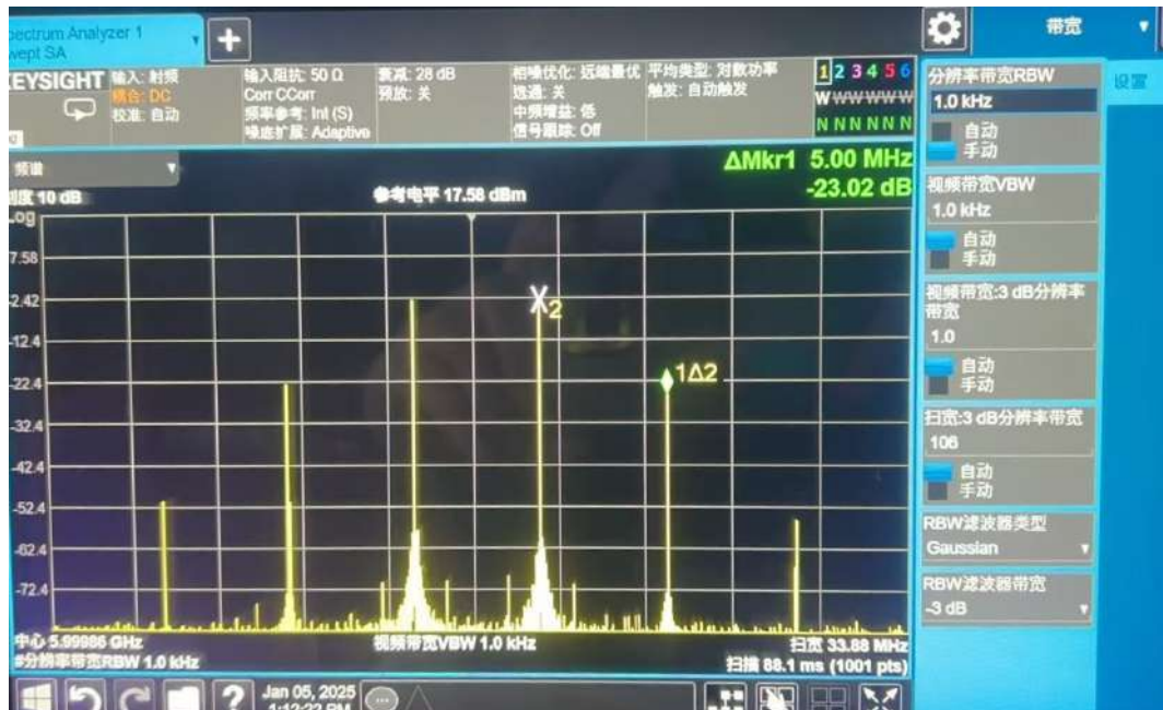
Figure 37 6.0GHz IMD3 Test Result
